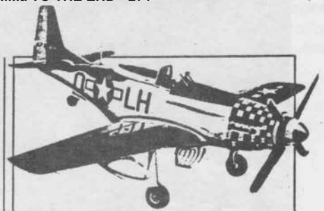
JOINT VENTURE The US P-51 Mustang fighter hail a British Rolls-Royce designed engine. Extra under-wing fuel tanks put eastern Germany within range, and a bubble canopy improved visibility.
