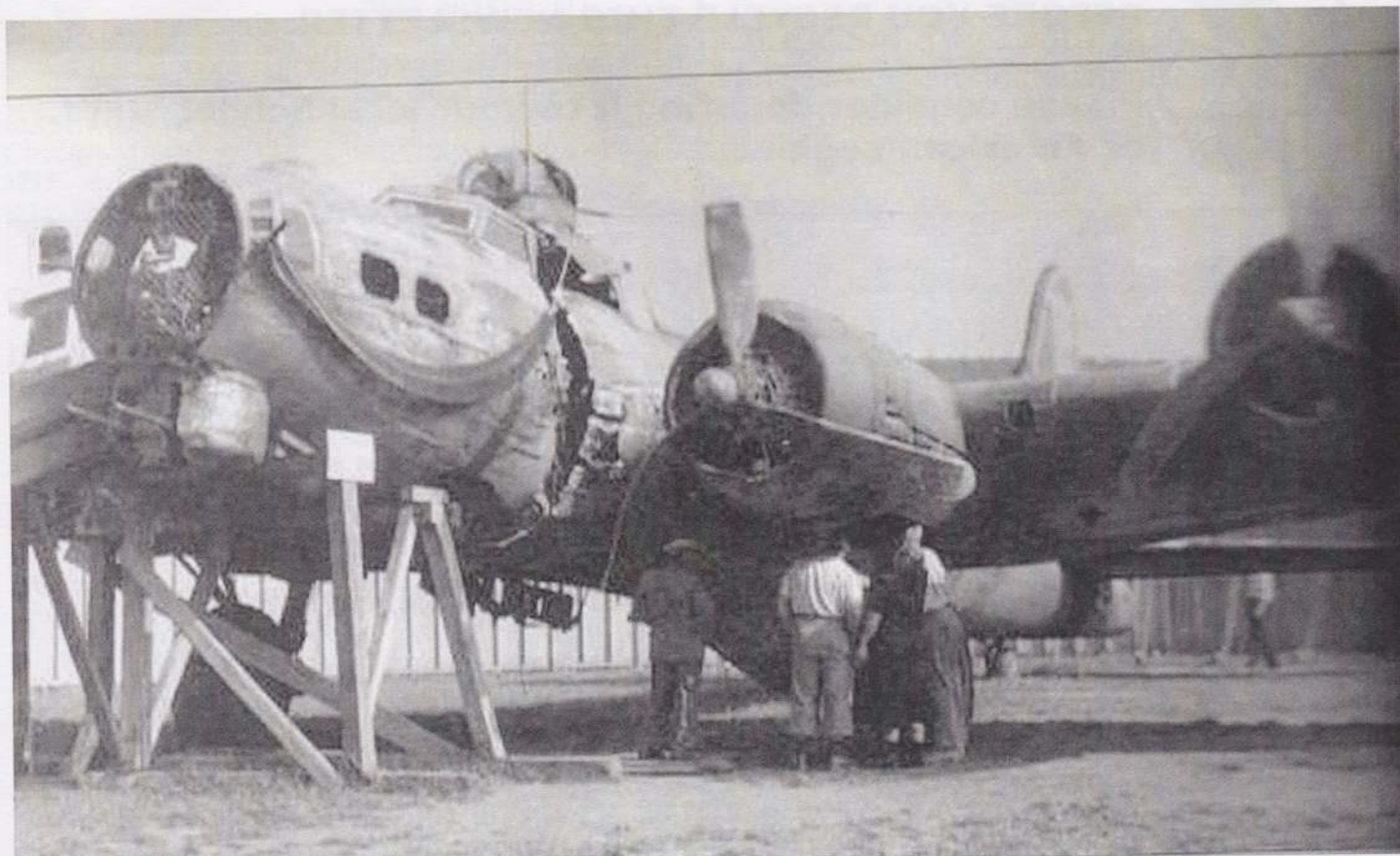
42-38160 "Lonesome Polecat" nose repair.
